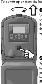
Twist the "Stop Button" red cap clockwise until the latch releases and the red cap springs upwards.
